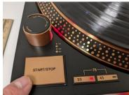
Select the **correct speed** (revolutions per minute) based on the vinyl record you have placed on the spindle. If you require 78 RPM speed press **BOTH** "33" and "45" at the same time.
